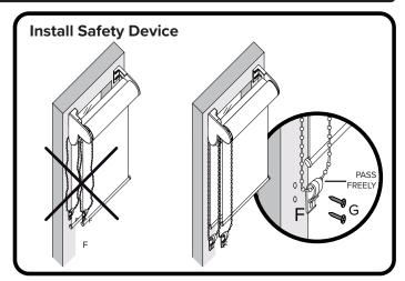
Lightly tension ball chain and fit tension device securely to Architrave/Wall. Allow enough play for chain to pass through device freely.
