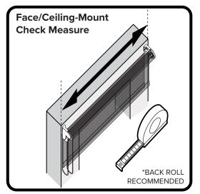
**Face Mounted** blinds are fixed to either: Architrave, Lintel/Wall or ceiling above the window frame. Measure width to cover opening as shown above.
