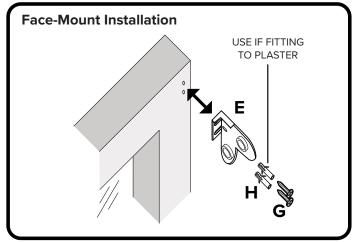
Secure to Architrave or Wall as shown above using screws provided. Use plaster plugs if fixing to wall.
