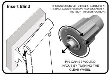
Insert mechanisms into tube on desired sides and insert into brackets. Pin mechanism can be wound in/out for easy blind removal & access to window.
