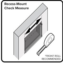
**Recess Mounted** blinds are fixed inside the window frame. Measure width to fill opening as shown above.
