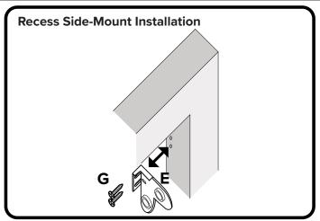
Secure inside window frame as shown above using screws provided
