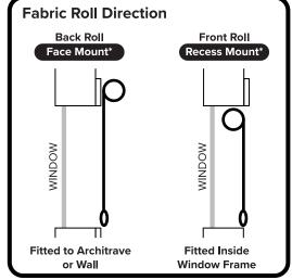
Fabric can be rolled from the front or back by simply flipping the entire roller tube.
