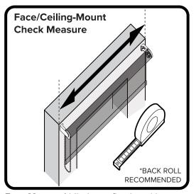
**Face Mounted** blinds are fixed to either: Architrave, Lintel/Wall or ceiling above the window frame. Measure width to cover opening as shown above.
