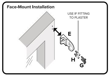
Secure to Architrave or Wall as shown above using screws provided. Use plaster plugs if fixing to wall.
